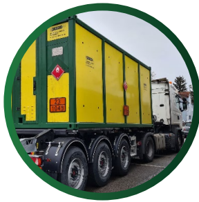
TPED container attached to a truck
