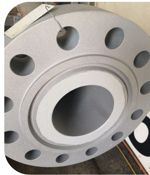
Pipe after inside coating.
