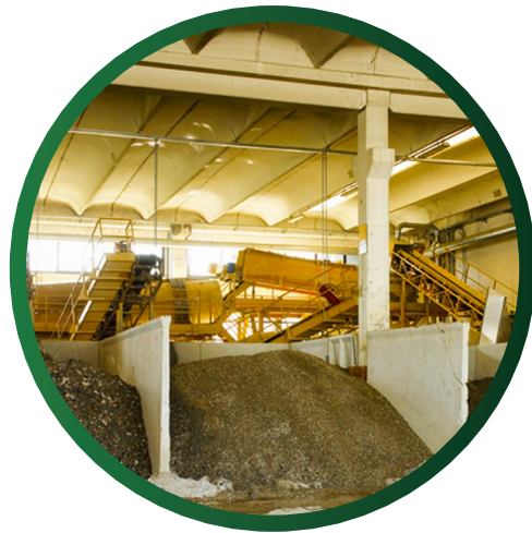
Woltank's soil washing plant with different types of soil separated.
